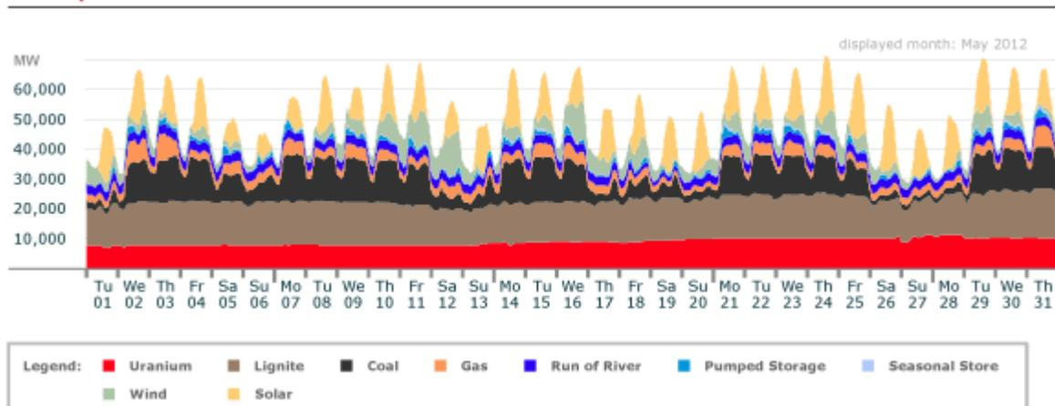
This next graph (below) shows the last week of May in a bit more detail. Those peaks now occupied by solar are what the gas-fired generators would normally expect to occupy. Not only is solar muscling these generators out of the system, they are also causing a significant reduction in wholesale prices – the merit order effect.
